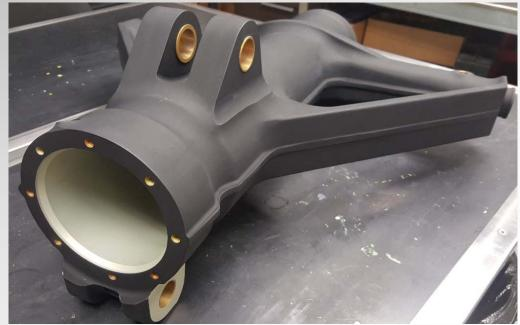
Landing Gear Housing for the CH-53
