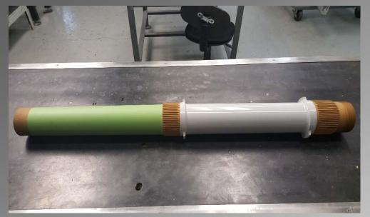
Torque Tube Assembly for the 767
