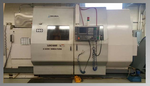
*The maximum CNC Lathe Capacity is 32" Dia. x 120" Length.*
