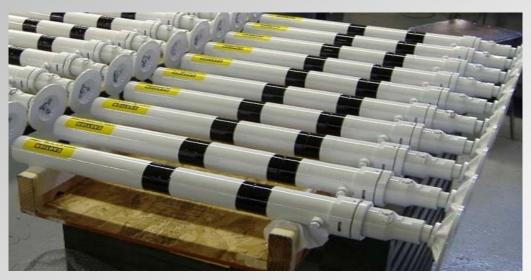
Rammer Cylinder Assembly for M -901 Tank
