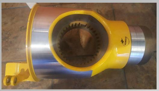
Trunnion Assembly for KC-135 Landing Gear
