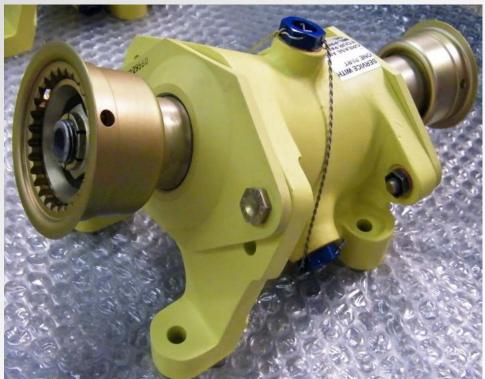
Torque Converter Assembly
